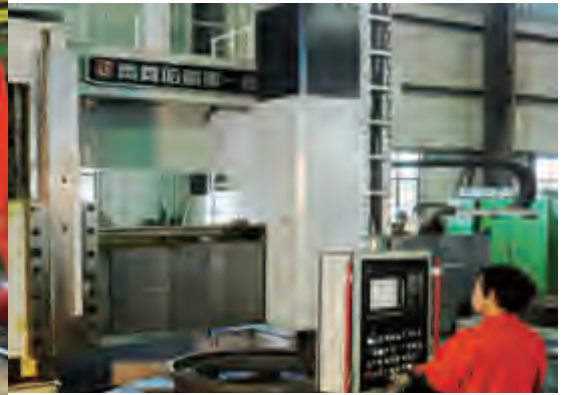
DVT250 × 16/16Q-NC 数控双柱立式车床 DVT250 × 16/16Q-NC CNC double column vertical lathe
