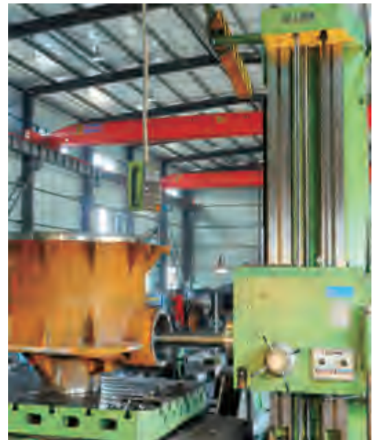
沈阳第一机床的 TPX6213×56 数控落地铣镗床 TPX6213 × 56 CNC Boring and Milling Machine from Shenyang NO.1 Machine Tool
